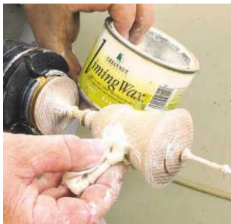
▲ Pic.32 Rub the liming wax into the grain using a rag. Make sure the grain is filled up, protecting your hands with some disposable gloves as it does get under your fingernails
